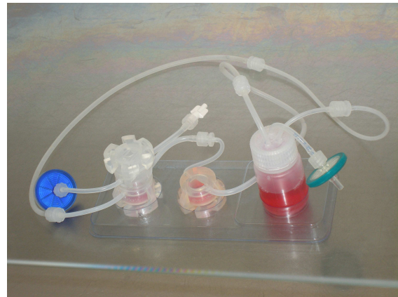
Obr. 3: Manipulace s „Quasi-Vivo inter-connected cell culture systems“.
